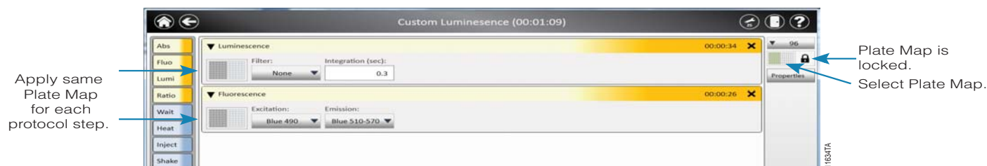
Figure 6. When the plate map is locked, the map is applied to each step of the protocol.
