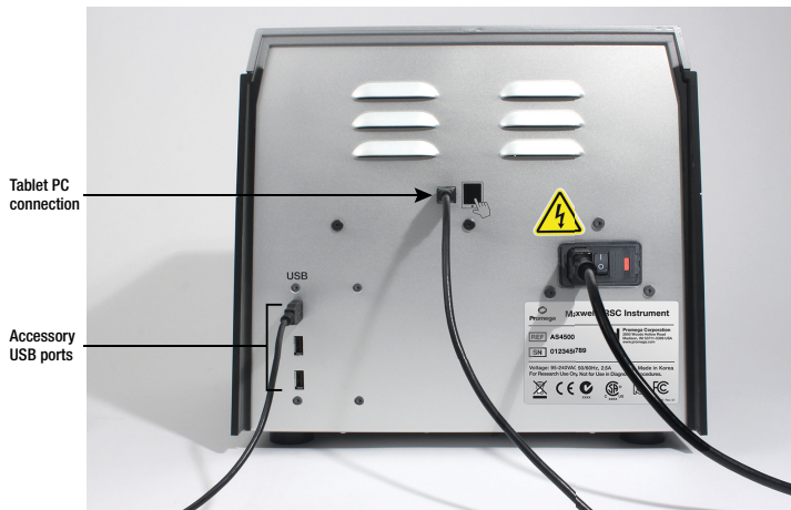
Figure 11. Connecting the Tablet PC to the back of the Maxwell® FSC Instrument.
