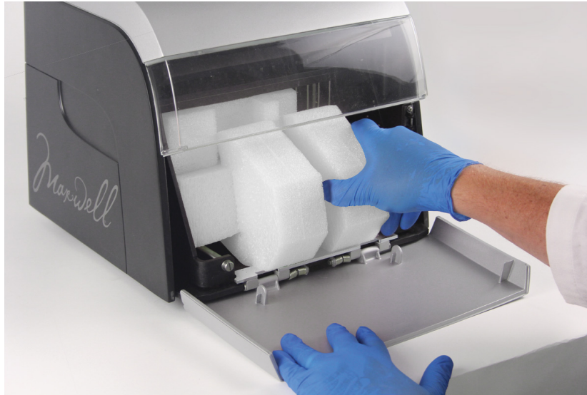
Figure 68. Placement of die cut foam in the Maxwell® FSC.
