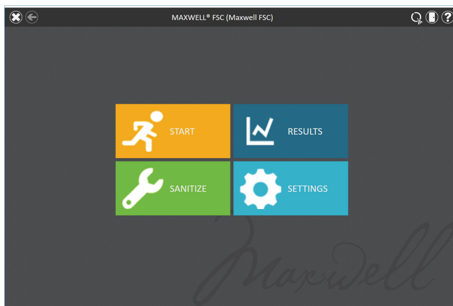
Figure 52. Maxwell® FSC ‘Home’ screen. When the Quantus™ Fluorometer is correctly connected to the Maxwell® FSC, the “Q” logo is displayed in the upper right corner of the title bar.
