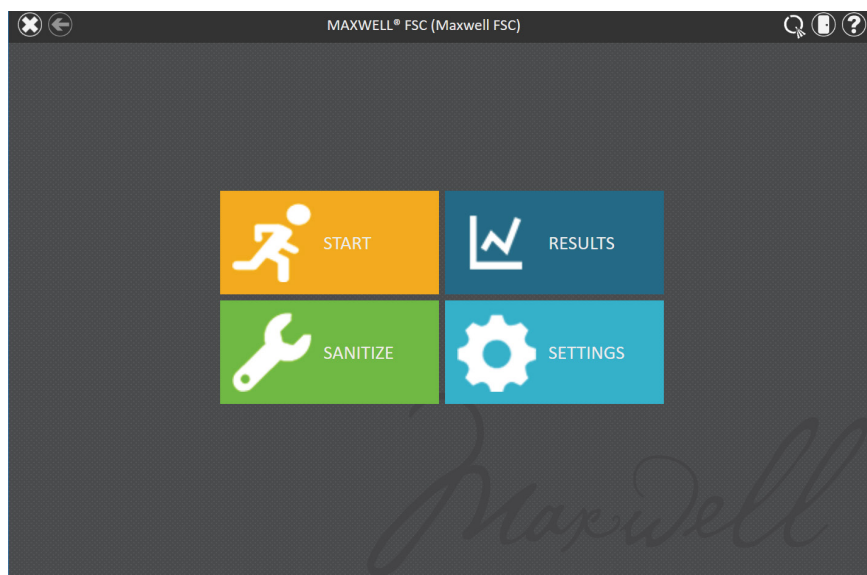
Figure 61. Maxwell® FSC 'Home' screen. Selecting Results opens the Maxwell® FSC 'Results' screen from which extraction reports from all method runs can be viewed.
