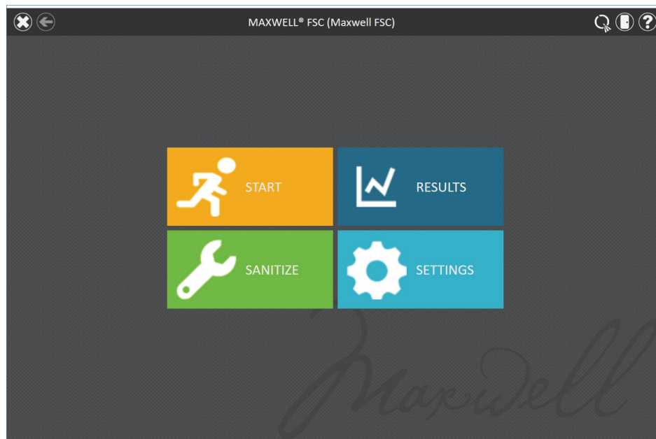
Figure 64. 'Home' screen. Selecting the Sanitize button begins the process for UV treatment of the Maxwell® FSC Instrument.
