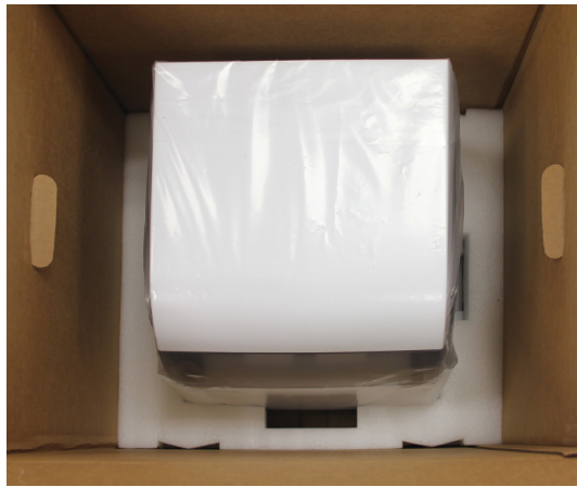
Figure 69. Repacking the Maxwell® FSC. Maxwell® FSC Instrument in the correct orientation in the box (A). Foam packing on top of box (B).
