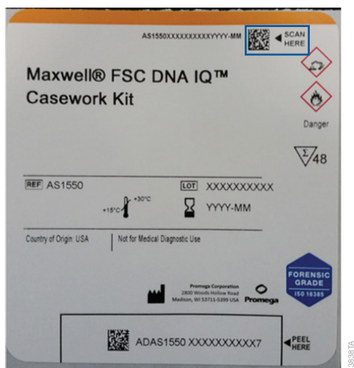
Figure 38. Kit label indicating bar code to scan. Shown in the blue box is the bar code to scan on the kit label for starting a purification run.
