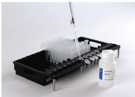
Figure 2. Setup and configuration of the deck tray(s). Elution Buffer is added to the elution tubes as indicated. Deck tray shown is from the Maxwell® CSC Instrument (Cat.# AS6000).
