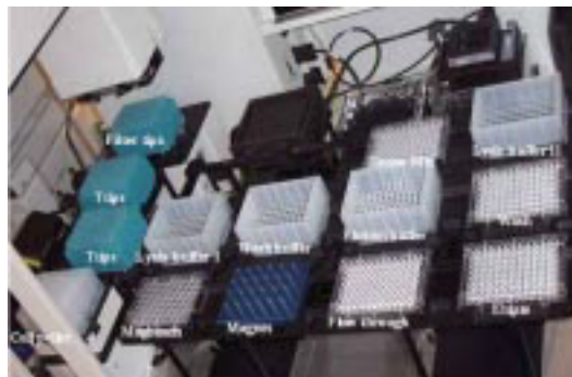
Figure 2. The position of containers on a Biomek® FX deck. The entire purification is performed on the deck of a Biomek® FX instrument. The flowthrough and wash can be collected (optional) or discarded to waste.
