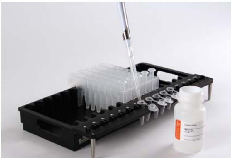
Figure 1. The RSC plunger is placed in well #8 of the cartridge (the well closest to the Elution Tube), and lysates and Lysis Buffer are placed into well #1 of the cartridge.
