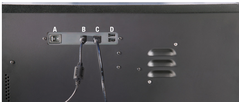
Figure 6. The back of the GloMax® Navigator Instrument. A. On/Off switch. B. Power connection. C. USB port to connect to Tablet PC. D. Two USB ports to attach an external USB flash drive, USB hub or Bar Code Reader..
